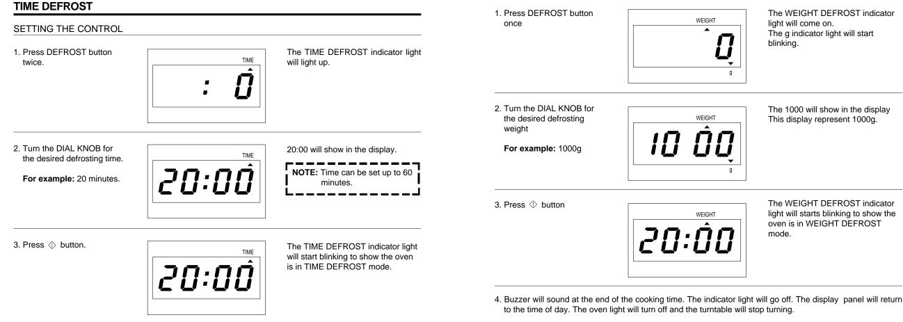
4. Buzzer will sound at the end of the cooking time. The indicator light will go off. The display panel will return to the time of day. The oven light will turn off and the turntable will stop turning.
